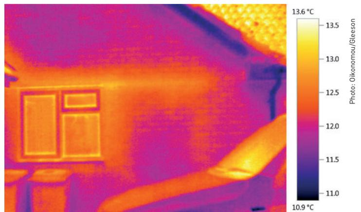
Thermal image showing incomplete cavity wall insulation around window
