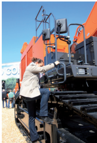
Unpractical access for small operators.
