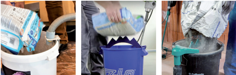
FIGURE 18: Extraction devices for buckets
