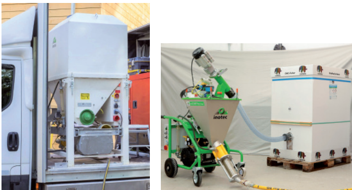
FIGURE 19: One-Way container on the pump truck or with mortar pump
