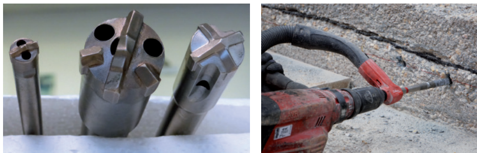
FIGURE 14: Tips of extraction drills and extraction drill with extraction socket
