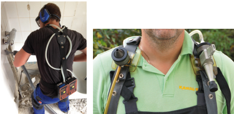
FIGURE 5: Two pumps on the belt of the employee; the filters are attached above the chest
