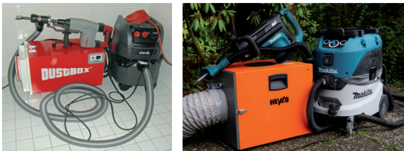
FIGURE 7: Low-dust equipment for a construction crew
