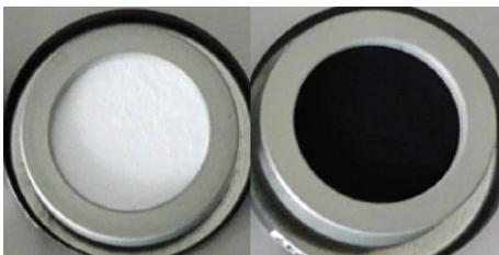
FIGURE 6: Filter of a Diesel exhaust measurement in the trench; left: new filter, right: filter after 30 min.
