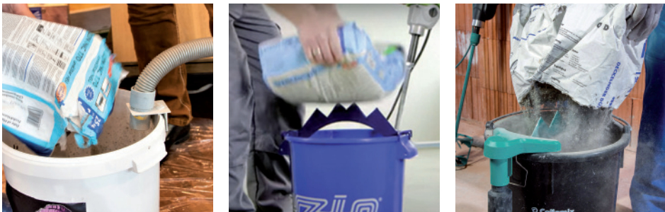
FIGURE 18: Extraction devices for buckets
