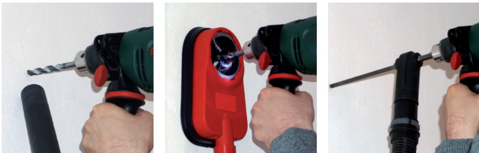
FIGURE 12: Left – This is how it is known – the vacuum cleaner nozzle is held under or next to the drill hole; middle – with vacuum cleaner adapter; right – with extraction drill
