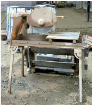
FIGURE 9: The mud under the stone saw dries and leads to dust
