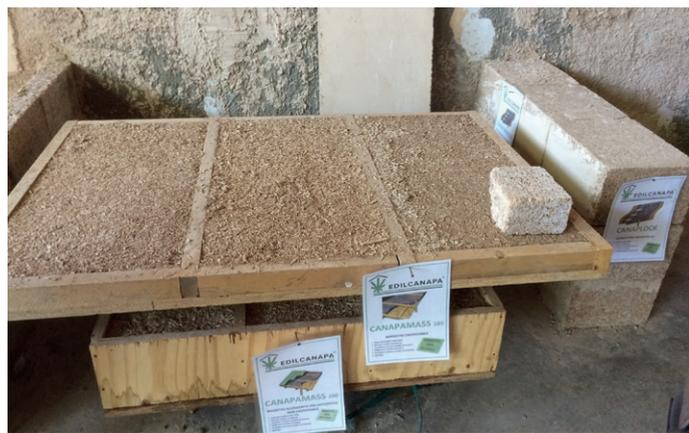
Hemp and lime based green building component, experimented with in CEFME-CTP training centre
